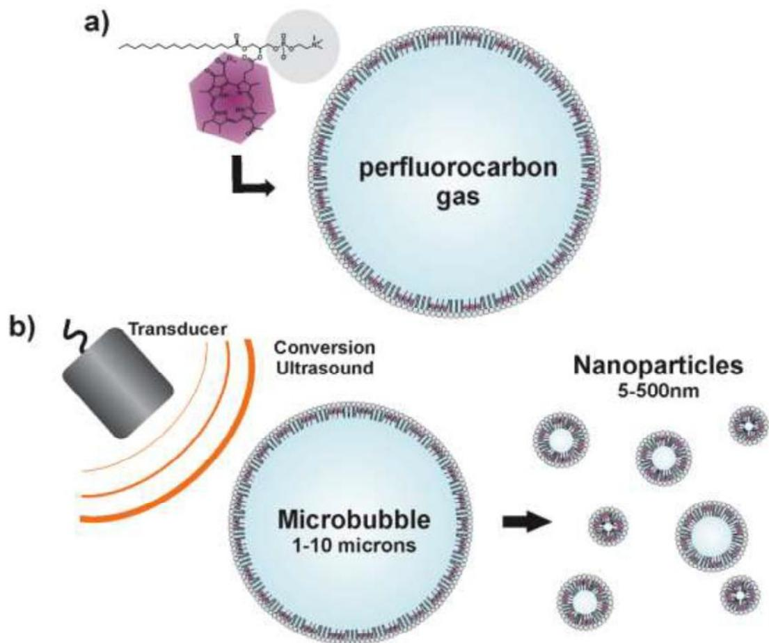
**Figure 1.** Schematics of porphyrin microbubbles (pMBs) and their micro-to-nano conversion. a) pMBs consist of a BChllipid shell encapsulating perfluoropropane gas. b) Conversion of pMBs to porphyrin nanoparticles (pNPs) via sonication with low frequency, high duty cycle ultrasound (conversion ultrasound).
